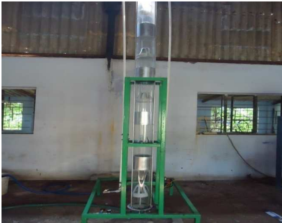
Fig.3 System Design of Water scrubber
