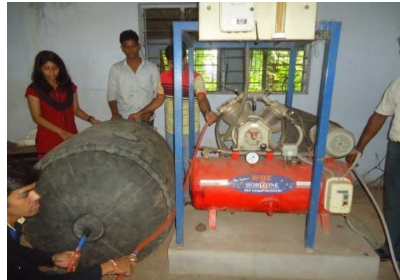
Fig.5 Two stage compressor and pressure vessel
