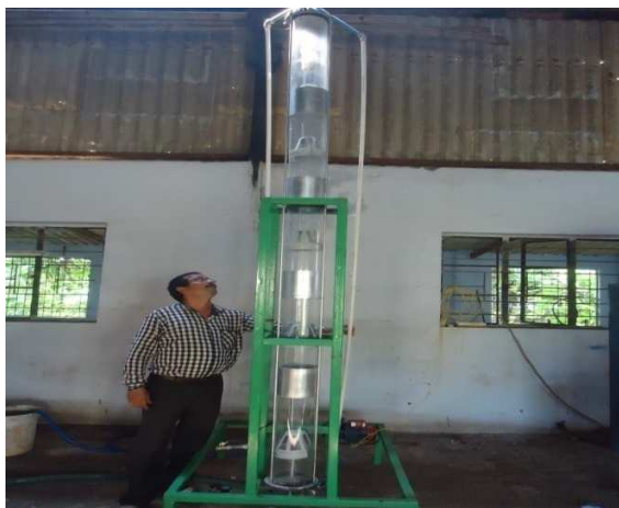
Fig.2 Water scrubber for biogas upgradation.
