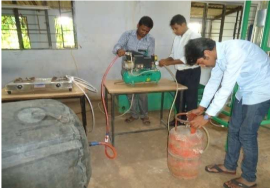
Fig.6 Storage of enriched biogas in LPG cylinder
